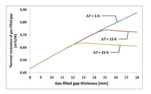
Fig. 1 Heat transfer through argon layer depending on the thickness of the gas layer and glass pane temperature difference [11]
