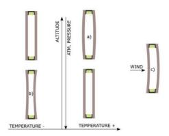
Fig. 2 Forms of IGU deformations
