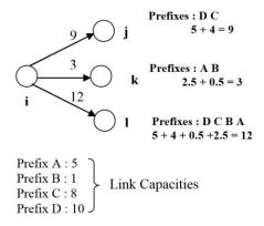
Fig. 3 (a) Subset split method - Simplified network
