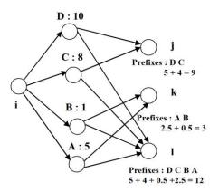
Fig. 3 (b) Subset split method – Complete flow from source "i" to destinations 'j', 'k' and 'l'
